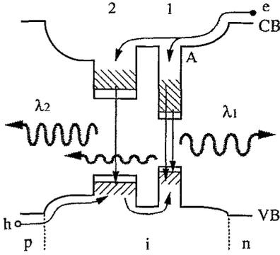
FIG. 1. Schematic band diagram of an ADQW LD. The shaded regions in the wells indicate the accumulated carriers.
