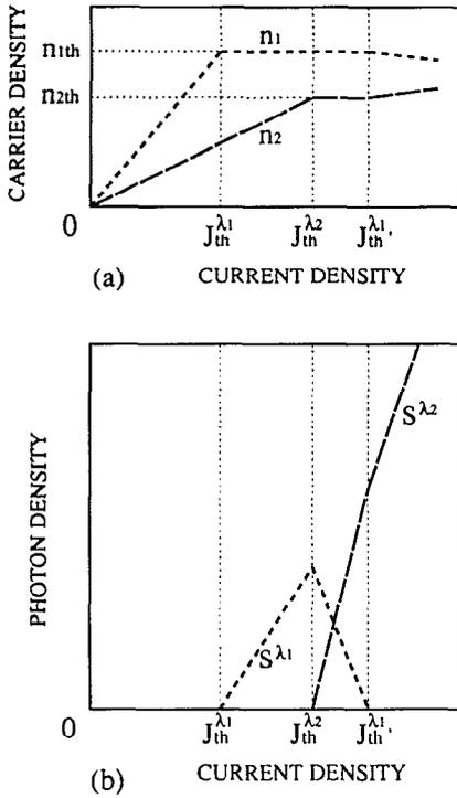
FIG. 2. Schematic plots of (a) the carrier densities and (b) the photon densities, as functions of the current density.
