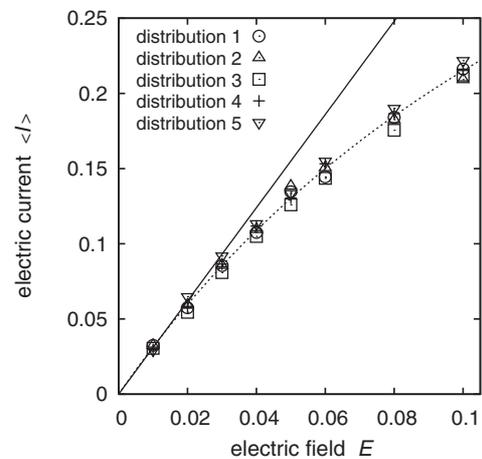
Fig. 2. Time-averaged electric current for various impurity distributions, plotted against an external electric field  $E$ . The values of parameters are the same as those in Fig. 1. The solid line is a straight line obtained from data for small  $E$ , and indicates a linear response. The broken line represents  $\sigma(E)EL_y$ , where  $\sigma(E)$  is given by eq. (4).
