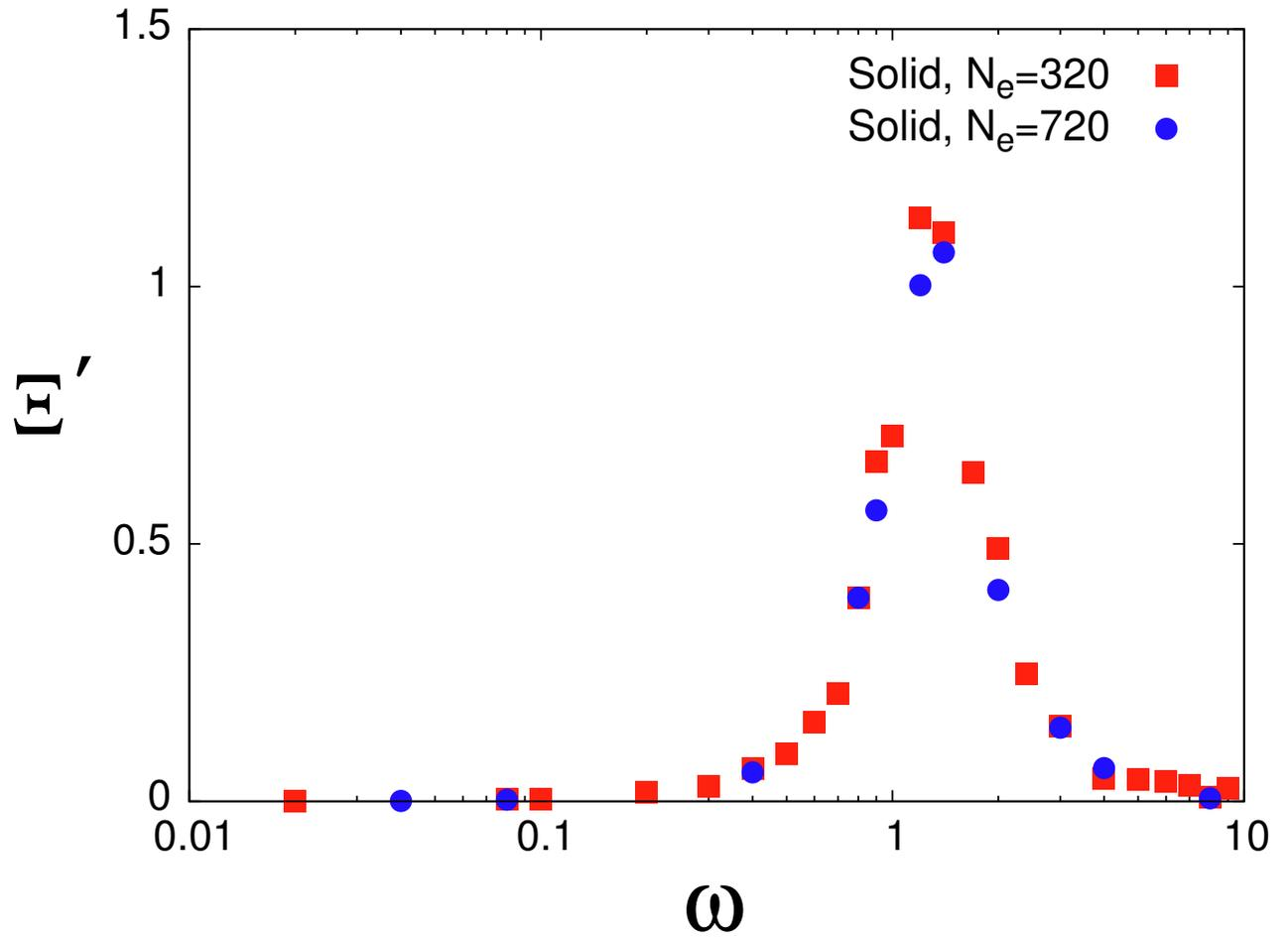
FIG. S3. The real part  $\Xi'(\omega)$  of the admittance for the solid phase, with  $N_e = 720, N_p = 360, N_i = 180, (L_x, L_y, L_z) = (18, 18, 15)$  (blue circle), and with  $N_e = 320, N_p = 160, N_i = 80, (L_x, L_y, L_z) = (15, 12, 12)$  (red square).
